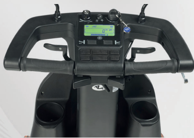
Redesigned tiller with onboard computer, LCD speedometer and two cup holders
